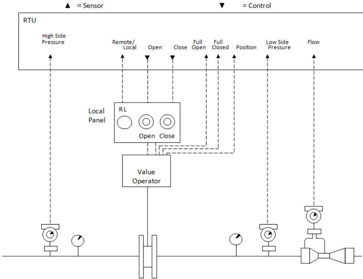
**Figure 3. Typical Control Valve controls and instrumentation**
