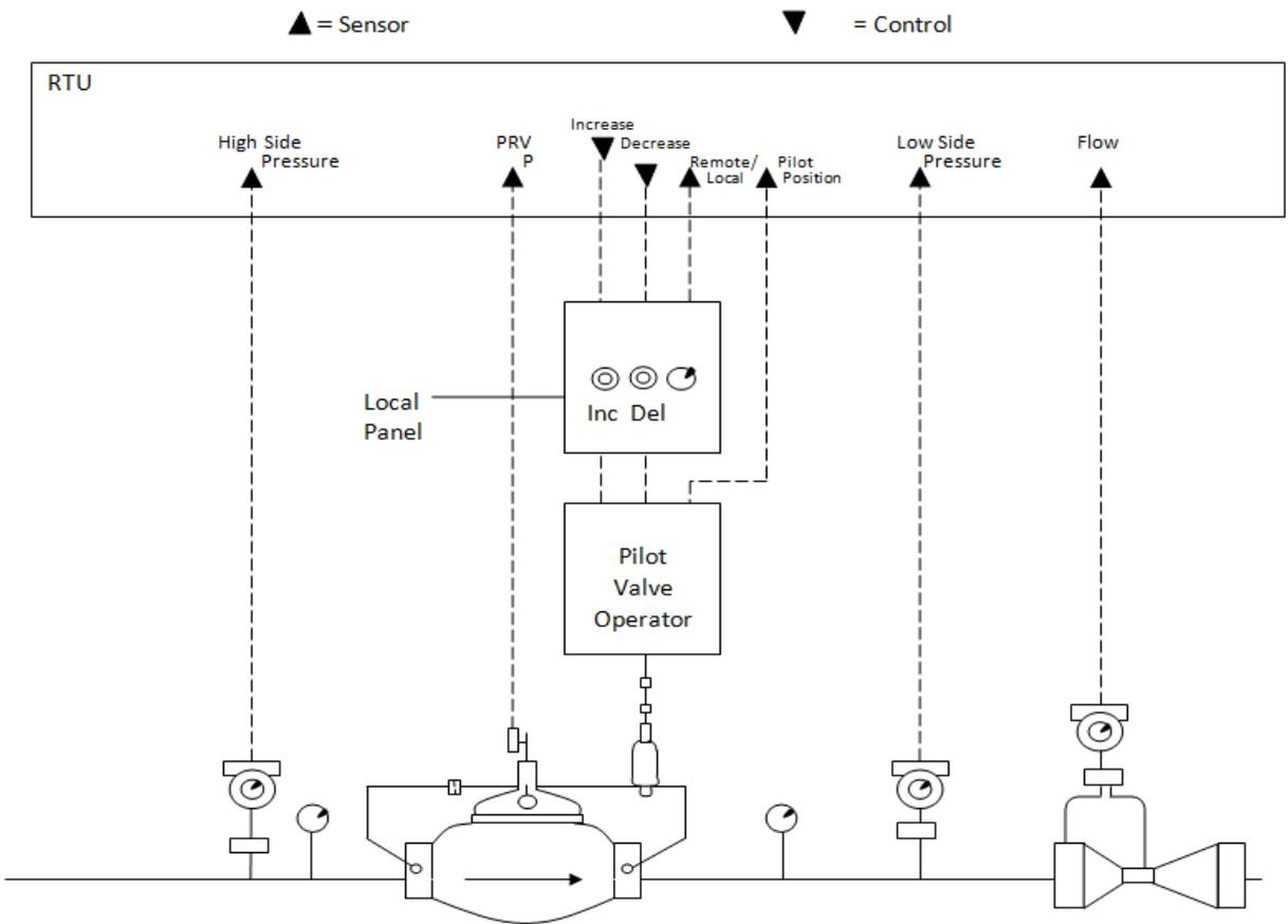
**Figure 2. Typical PRV controls and instrumentation**
